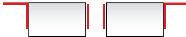
Angle Flat Bumpers Designed to have one side welded to the vertical curb angle and the other side bolted to the wall
