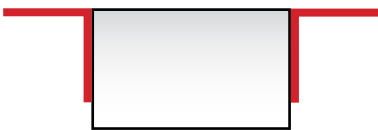
Angle Angle Bumpers Designed to have both sides bolted to the wall
