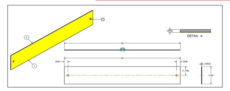
The bumper guide strip improves visibility when backing up to a loading dock. The bumper guide strip highlights the bumper area to the left and right of the dock doors providing a clear drive line for the truck backing up.
