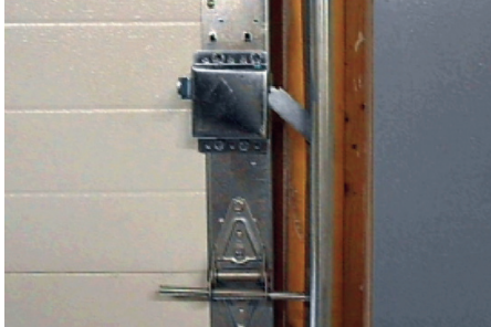
Traditional lock under pressure fails
